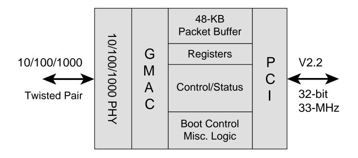
The Altima **AC1002** 10/100/1000 Gigabit Ethernet Controller is a highly integrated low-power CMOS silicon solution. It provides a complete triple-speed solution for 32-bit PCI v2.2. The on-chip, 48-KB packet buffer provides optimum performance for workstation/desktop applications.
