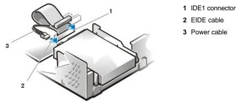
9. If it is not already connected, connect the blue end of the EIDE cable to the IDE1 connector on the system board.
