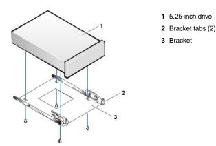
d. To further ensure proper positioning of the drive in the bracket, insert and tighten all four screws in the order in which the holes are numbered (the holes are labeled "1" through "4").
