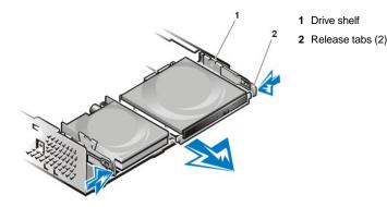
To remove the drive shelf from the chassis, perform the following steps:
