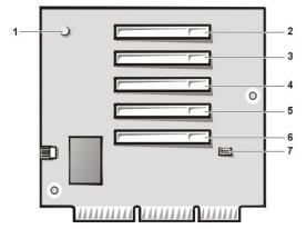
Figure 8. Mini Tower Chassis PCI/ISA Riser Board
