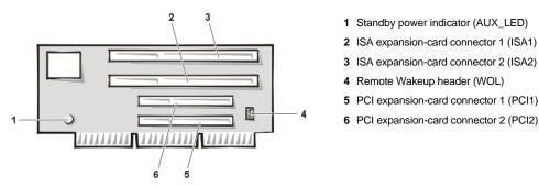
VI NOTE: ISA expansion-card connector 1 and PCI expansion-card connector 2 share an expansion slot; only one of these two connectors can be used.
