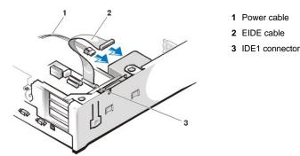
10. If it is not already connected, connect the other end of the EIDE cable to the IDE1 connector on the system board.
