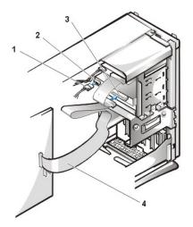
Connect the interface cable to the system board.
