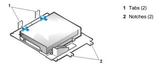
4. Lift the 5.25-inch drive bracket straight up and out of the chassis (see Figure 5).
