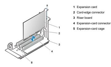
Figure 12. Installing an Expansion Card in a Midsize Chassis
