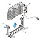
1 Pin-1 corners of chip and socket aligned
