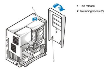
3. While you press the tab release, tilt the bezel away from the chassis, disengage the two retaining hooks at the bottom of the bezel, and carefully pull the bezel away from the chassis.
