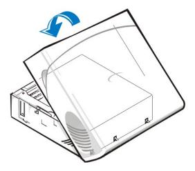
Figure 5. Replacing the Low-Profile or Midsize Computer Cover
